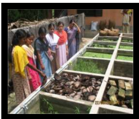
Fig.2a: Coconut husk kept soaked in water in tank before cocopeat production
